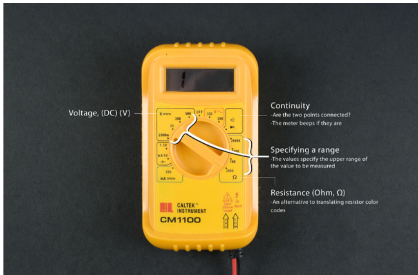
Figure 1-26. The most common functions of a multimeter
