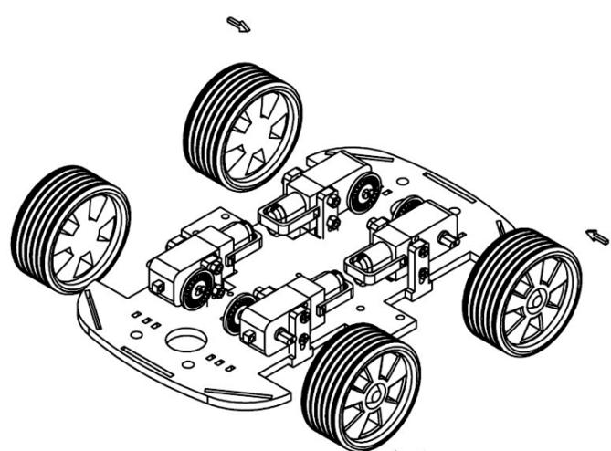
Step4: Hold tight and insert the motor (protection fastener) to the wheel.
