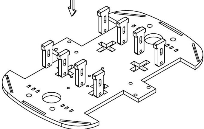
Step1: Insert the fastener into the chassis after tearing off the yellow protection wrap of the chassis, the fastener and the code wheel.
