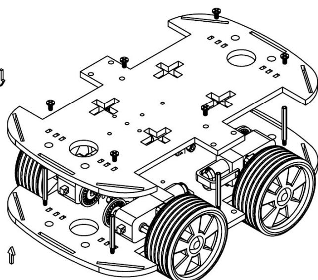
Step5: Insert the spacer, insert the screws from the downside and tighten them from the upper side. Installation completed.
