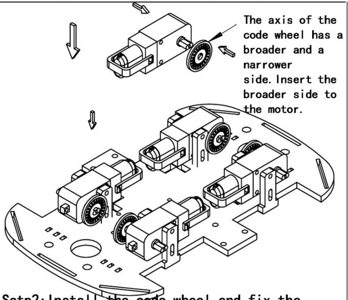
Step2: Install the code wheel and fix the motor to the chassis. (Attention:the copper sheet of the leading wire of the motor should face outward, the same side of the wheel)
