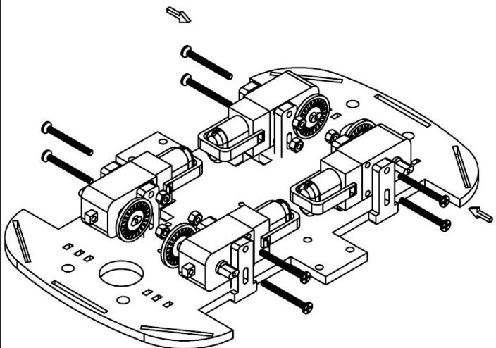
Step3: Fix the motor to the chassis, then insert and tighten the screws.
